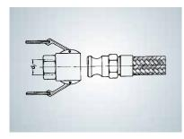
This quick release coupling stands out particularly through easy handling, quick mounting, robust design work and a long service life. In order to complete the coupling process, the two halves of the coupling are put together and securely connected with each other by applying both cam levers. As there is compression of the inserted seals rather than a turning movement when coupling up, the connection can be completed without damaging the hose by twisting.
