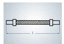
The following guidelines apply for measuring the length of the individual hose types:
