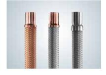
Corrugated hoses are mechanically formed from seamless or longitudinally welded tubes and are available in a variety of wall thicknesses, material types and packaging from DN 4 to DN 300. These are used to convey pressurised fluids and fluids in a vacuum in an absolutely leak-tight manner. The hoses are used to compensate movements, thermal expansion and vibrations within piping systems.
